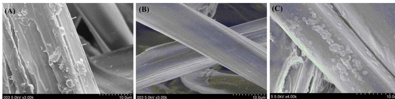
Figure 6. Scanning electron microscope images of silk fibers before and after soaking in DMF for 24h. (a) Silk fibers prepared by physical adsorption of P1, (b) Silk fibers by P1 adsorption after soaking. (c) Silk-P1 after soaking in DMF. [Color figure can be viewed in the online issue, which is available at wileyonlinelibrary.com .]
